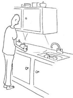
Solution: To avoid shadow and provide equal light, recessed dimmable led down lights provide the solution for both style and running costs. A less effective but practical alternative is to look at a multi head fitting on a bar which will cover an area wider than the location of the wiring.
